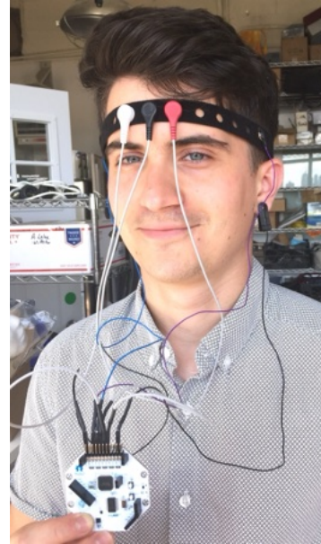
Figure 5: OpenBCI headband setup (OpenBCI Docs, n.d.)
